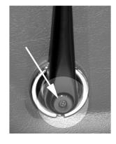
(forward of neutral or back of neutral upright position). Return the throttle to idle position, and the transmission lockout will automatically reengage the transmission in neutral position.
