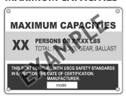
In compliance with United States Coast Guard Regulations, Moomba Boats meet or exceed all safety standards designed for recreational boats. To ensure safe handling and performance, each Moomba boat displays a maximum capacity sticker (see sample), stating the maximum passenger weight load allowable.
