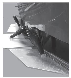
The multisport wakeplate allows the driver to control the running attitude of the boat.
