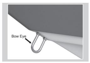
The bow eye is located at the front of the hull below the rub rail. It is the point of attachment to lead the boat onto the trailer and to secure the boat to the trailer or to a tie-off when docking.
