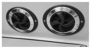
The boat heater is a forced air heater that uses hot engine water as a heat source. To use the heater, simply turn the heater switch to the selected fan speed. In order for the heater to work, the engine must be at operating temperature. One of the features of the heater are the snorkel vents, which can be pulled out to direct heat to specific areas.
