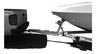
**NOTE:** If your hitch ball has an excessive flat spot on top, the latch may not engage properly. If the latch does not catch, check with your dealer or hitch installer before trailering.
