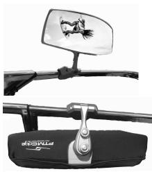
The rear view mirror is installed as a standard item. The mirror is adjustable so that it may be set for each driver.
