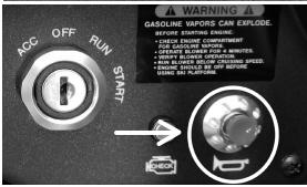
The Horn Switch is located on the switch panel to the left of the steering wheel.
