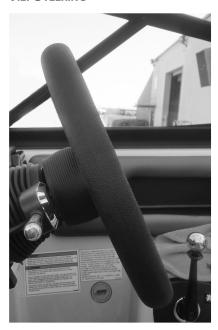
Tilt steering may be adjusted up or down in five different locking positions. To adjust, depress the tilt lever located beneath the bezel and move the steering wheel to the desired position. Release the lever to lock the wheel into place.
