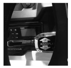
The Wakeplate switch controls the position of the center trim tab (wakeplate). The down position raises the stern of the boat and lowers the bow. The wakeplate helps shape the wake for surfing and wakeboarding.
