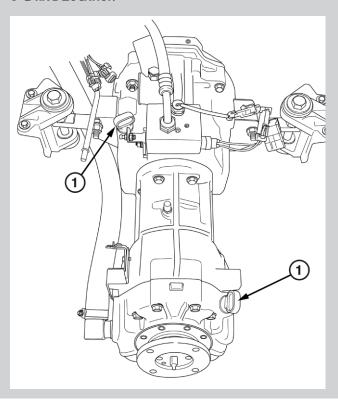
The fluid level can be checked by using the oil level dipstick, which is located on top of the V-Drive transmission. This unit's located under the center cushion of the rear seat. Pull out the cushion to access the transmission.
