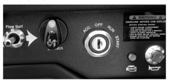
Located on the port side of the dashboard, the ignition switch has four positions. In the vertical position, the ignition is "OFF".
