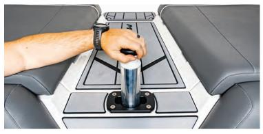
The ski pylon is only to be used to pull skiers. **DO NOT use the ski pylon to hoist the boat.** Only use the lifting rings for this purpose.
