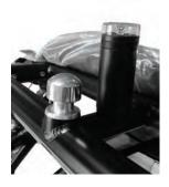
On boats equipped with factory installed towers, the 360° White Anchor/Running Light is mounted on the tower.
