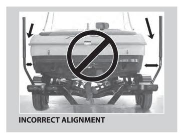
The distance between the boat and the wheel runner board should be about equal on both sides.
