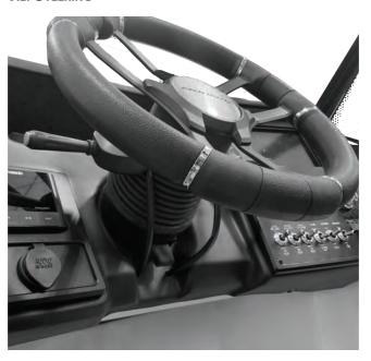
Tilt steering may be adjusted up or down in five different locking positions. To adjust, depress the tilt lever located beneath the bezel and move the steering wheel to the desired position. Release the lever to lock the wheel into place.
