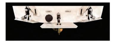
The multisport wakeplate allows the driver to control the running attitude of the boat.
