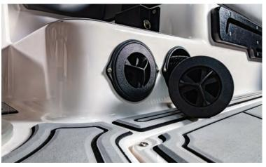
The boat heater is a forced air heater that uses hot engine water as a heat source. To use the heater, simply turn the heater switch to the selected fan speed. In order for the heater to work, the engine must be at operating temperature. One of the features of the heater are the snorkel vents, which can be pulled out to direct heat to specific areas.
