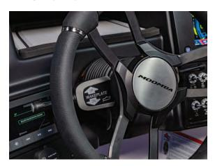
The Wakeplate switch controls the position of the center trim tab (wakeplate). The down position raises the stern of the boat and lowers the bow.
