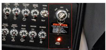
Located on the starboard side of the dashboard, the ignition switch has four positions. In the vertical position, the ignition is "OFF".
