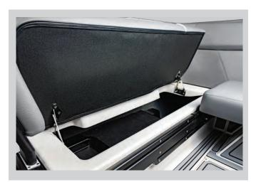
It is important to provide for the drying of all upholstery and carpet after each use of the boat. Open all storage compartments and slide all removable cushions out about an inch to allow air to circulate behind. If cushions are wet, turn them up at an angle as shown above to promote drying.
