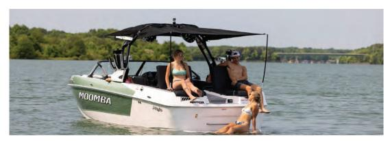
The optional tower bimini is a deployable sun shade that can be used when the boat is running or sitting still. To deploy bimini, first remove bimini boot. Next, remove pins from bimini arm and fold bimini frame out and secure to bimini arm with clips. Next, unroll bimini and attach bimini to tower using Velcro strips. You can adjust tension in the bimini by how tight you attach Velcro strips. To fold bimini back into storage position, reverse installation instructions.
