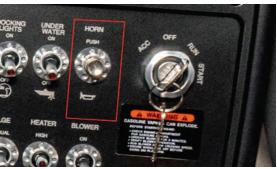
The Horn Switch is located on the switch panel to the right of the steering wheel.
