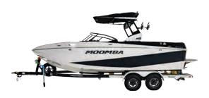
The trailer supplied with your Moomba model was designed especially for the boat with your convenience in mind. Please be sure that you have an appropriate tow vehicle before attempting to trailer your boat. Your vehicle must be capable of towing 4,500 - 6,000 lbs., depending on the model.
