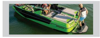
All Moomba models are equipped with a swim platform on the stern. The platform allows easy access to and from the water for boat passengers. It is recommended that all entries to and exits from the water be made from the platform to avoid accidents. (The fiberglass deck can become slippery when wet.)
