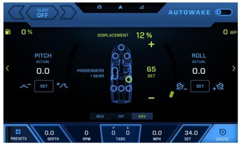
This page displays a graphical representation of where to move or place passengers or ballast to optimize the weight to pitch and roll ratio.
