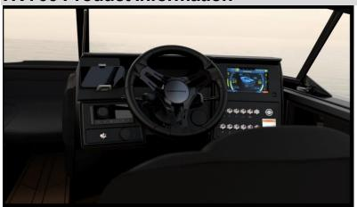
The Moomba® 7" Touch Screen 2023 display is designed for instrumentation and control on electronically controlled engines communicating via SAE J1939 and NMEA 2000. The display is a multi-functional tool that provides GPS tracking, AutoWake/Surf controls and ZeroOff®GPS Cruise control settings while enabling boat operators to view vital engine, ballast settings and service codes. Included with this solution is the HV700 Touch unit.
