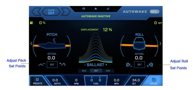
This page allows the manipulation of the pitch and roll values. Touch and adjust via the +
