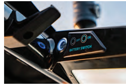
*E/PEX TOWER BATTERY SWITCH
