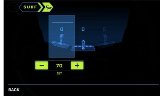
Because Surf Right is selected, the right tab is grayed out. Only the Center and Left tabs can be adjusted by touching the + or – buttons. The same procedure is reversed when surfing Left:
