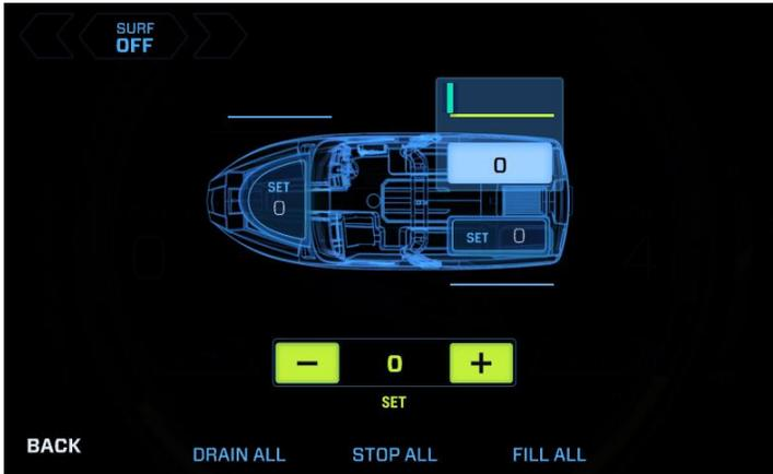
Ballast is used to add displacement to the craft to make the waves or wakes larger for specific watersports. This Moomba model is outfitted with one ballast bag located in the front, and two ballast bags located in the port and starboard sides of the rear. Touch the graphical level representation of one of the ballast settings on the main screen, and this screen will appear:
