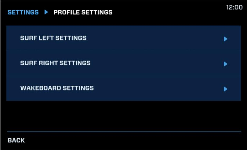
This settings screen will establish the speed, flow plate, wakeplate and maximum displacement settings for both left and right surfing and wakeboarding.
