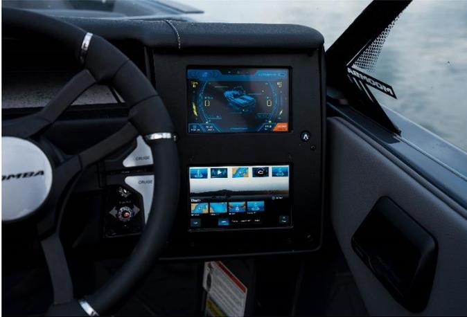
The Moomba® 7" Touch Screen 2024 display is a multi-functional tool that provides ZeroOff®GPS Cruise control settings and AutoWake/Surf controls while enabling boat operators to view vital engine, ballast settings and service codes. This solution includes the HV700 Touch unit which is designed for instrumentation and control on electronically controlled engines communicating via SAE J1939 and NMEA 2000.
