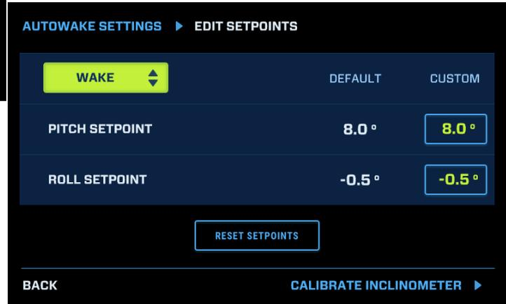
Touch the Custom Setting box for either Pitch or Roll, and the screen will change to be like the following:
