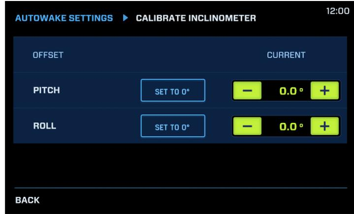
If the “current” number shows 0.0, then the inclinometer calibration has been cleared and needs to be calibrated.
