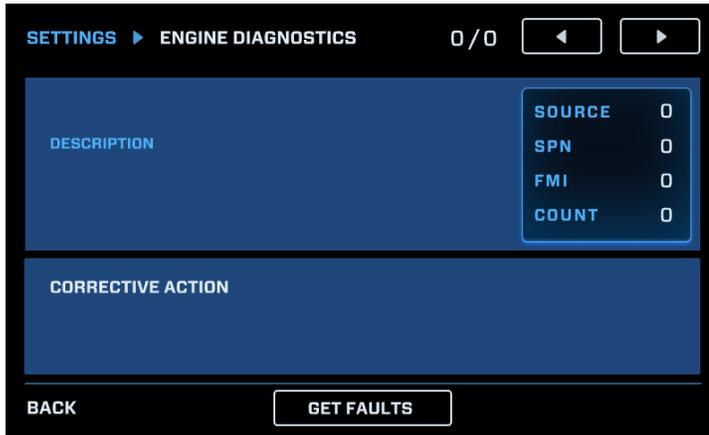
The engine's ECU is queried and displays feedback on any diagnostic codes that have been activated and stored in the ECU for service needs.
