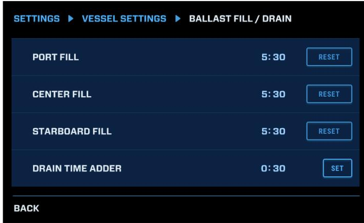
This screen establishes how long it will take for each of the ballast bags to fill or drain. Touch Reset to adjust a Fill time and the following will appear:
